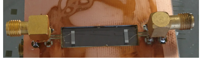
Fig. 4. SAW delay line for simulating the satellite motion by heating the piezoelectric substrate to induce acoustic velocity change and hence time of phase variations. The long delay line designed to induce sufficient delay variations when heating only induces minor losses since propagating a Rayleigh wave. The interdigitated electrodes visible on both ends of the propagation path free of electrodes, next to each SMA connector.
